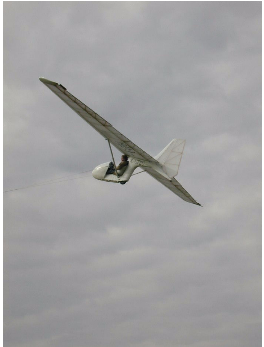
Mat Redsell takes his Monarch up on auto tow. This launch method is quite inexpensive. A strain gauge readout visible to the driver makes sure the line tension remains consistent. Photo by Bill Kuhlman taken during the May 2000 workshop.
